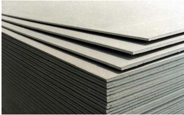
Figure 2 Strapping removed - sheets can slide off
